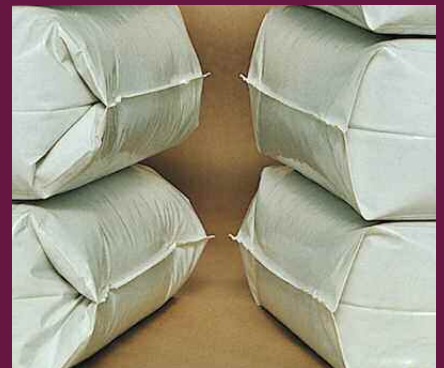
洁净、饱满的FFS袋子以及最小的对接焊缝 Compact, clean FFS bags with minimum welding seam
